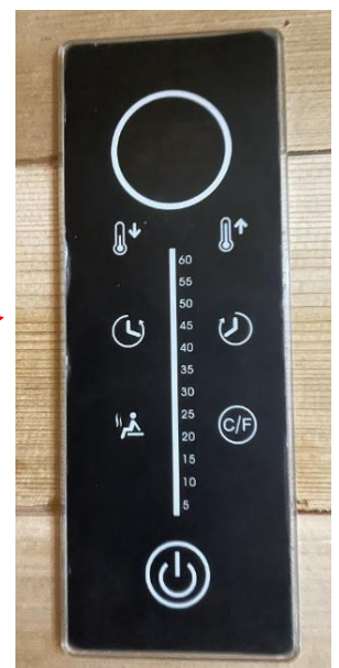
Sauna Control Panel has no Illumination
