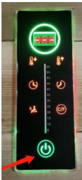
Sauna Control Panel is Illuminated
