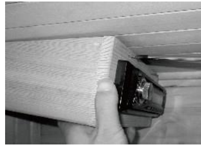
FIG-17 Screwing in the Radio Wood Housing
