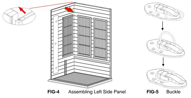
4. Latch the Left Side Panel with the Back Panel. The buckle has a guide tab that must be placed in the guide slot for alignment. When the Back Panel and the Side Panel is attached together on the floor panel, make sure all the buckles are latched. See FIG-5 **5.** Align the Right Side Panel with the Floor Panel's corresponding patterns; make sure the Right Panel fits flush into the Back Panel and latch together. **See FIG-6**
