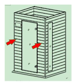
FIG-11 Assembling Front Panel
