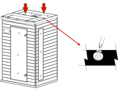
FIG-12 Installing Roof Cover
