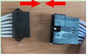
FIG-18 Connecting control panel connectors
