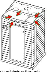
FIG-13 Slip cords/wires through corresponding holes
