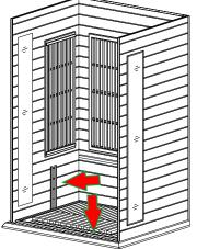
FIG-7 Placing Floor Heater
