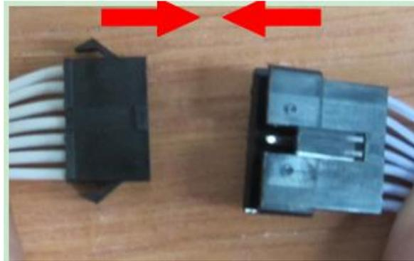
**FIG-18** Connecting control panel connectors
