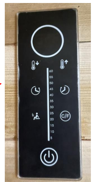
Sauna Control Panel has no Illumination
