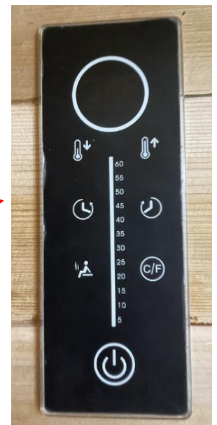
Sauna Control Panel has no Illumination
