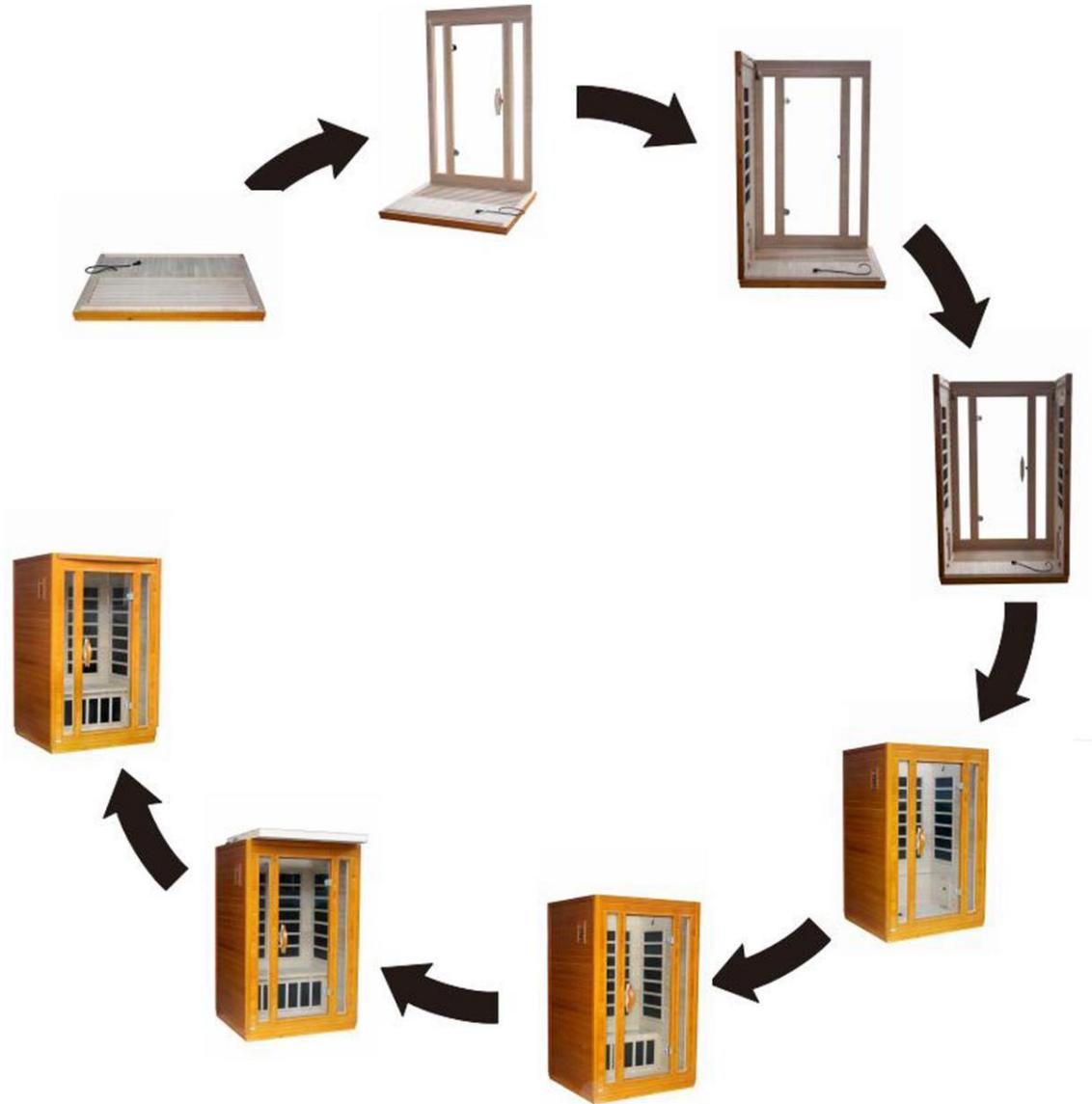
**\*The above assembly diagram is for a quick reference visual guide only. All sauna models are not shown. Parts and accessories may vary and are subject to change. Backrests are sold separately. We have found that starting the assembly process with the floor and front wall panel first may be the easiest, but it is not mandatory.**
