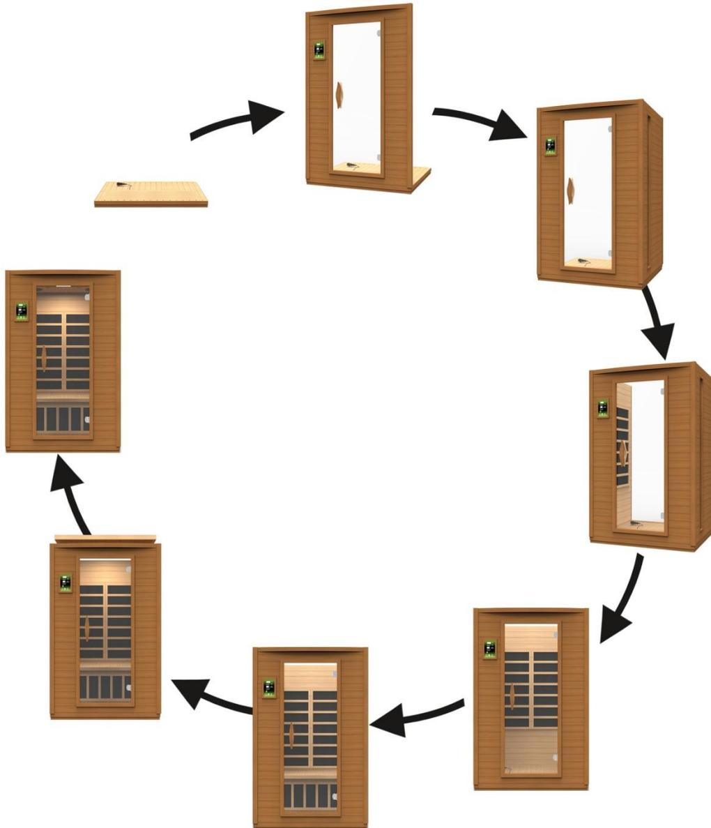
**\*The above assembly diagram is for a quick reference visual guide only. All sauna models are not shown. Parts and accessories may vary and are subject to change. Backrests are sold separately. We have found that starting the assembly process with the floor and front wall panel first may be the easiest, but it is not mandatory.**
