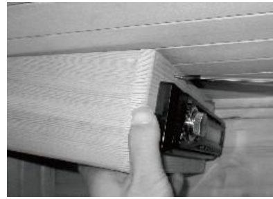
FIG-17 Screwing in the Radio Wood Housing
